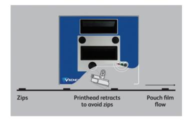
A simple software setting can retract the thermal transfer printhead up to 4.5mm
